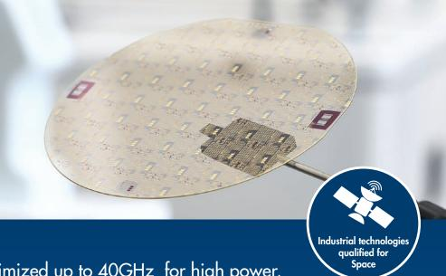
GH15 GaN process is optimized up to 40GHz for high power, high PAE and high linearity.
